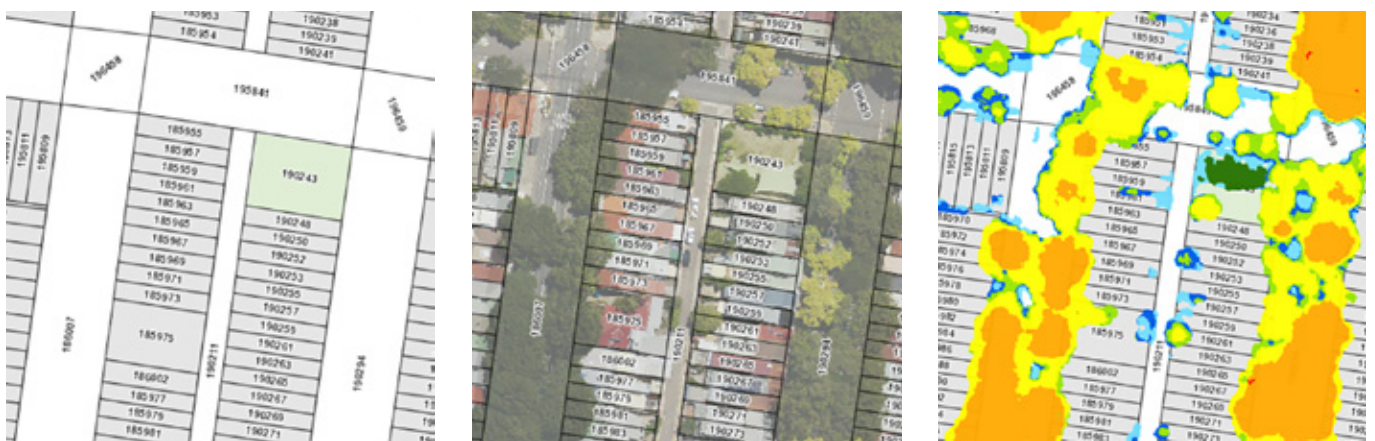
Figure 32: Example of street, park and property land parcels, each with a unique site code identifier overlaid on aerial image and aerial acquisition of vegetation height strata.
